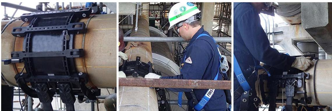
FIGURE 8. CUI pipe inspection in an alkylation unit at an oil refinery.
